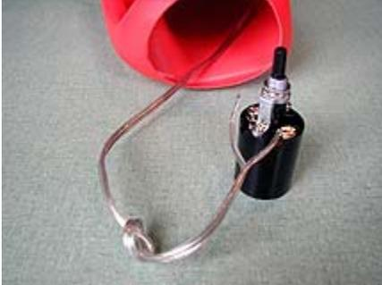
10. Now, thread the lamp cord through the hole on the bottom which is closer to the handle side of the container. Once it is through the base, tie a simple knot about 4 inches or so down the cord – this keeps the cord from slipping out of the hole. Then, attach each wire end of the lamp cord to the bottom of your socket.
