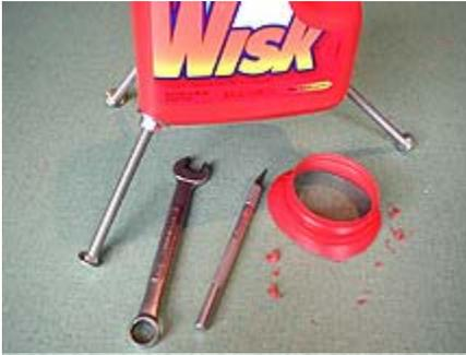
8. Once you have all the legs installed, place the container on its new feet and see how it stands. Adjust the length of each leg by screwing in the legs until the container sits level on the table. Then, with your wrench, tighten each nut on the outside of the container while holding the carriage bolt with your other hand until they are fastened securely. You are almost done!
