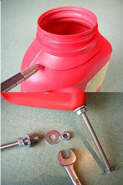
5. Now you will need to cut off the top of your container. Carefully take your x-acto knife and slice through the plastic just beneath the threaded 'cuff' of the top. The size of this opening is up to you but make it big enough so you can just fit your hand in to make the assembly easier in the steps to follow.
