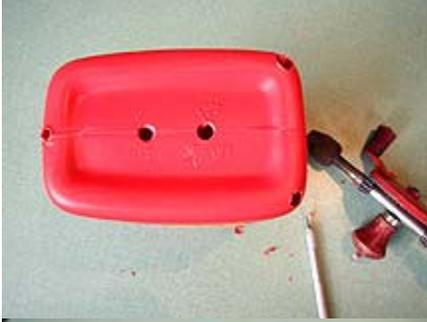
4. You will need to drill two more holes on the bottom, one for the lamp socket switch and the other for the lamp cord. Drill the lamp socket hole first placing it directly under the center of the top opening (the spout) of the container. Then, drill the other hole about an inch or so beside it (this hole resides more underneath the handle). Use your x-acto knife to carefully clean up the newly drilled holes, trimming away any unwanted plastic.
