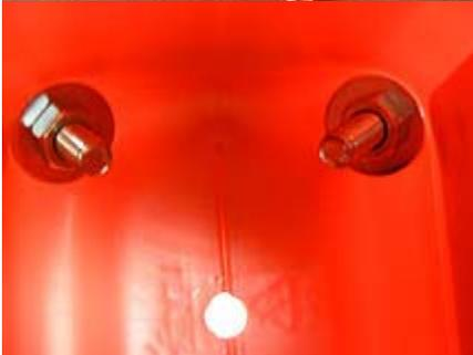
7. Reach inside the container and place a washer and then a nut on the end of the bolt and finger tighten each nut until snug. Repeat steps 6 and 7 for the remaining two legs
