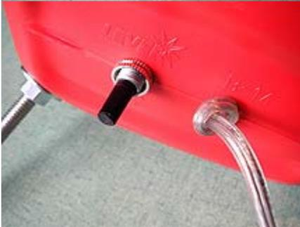
11. Remove the nut from the end of the socket and then reach inside the container and stick the end of the socket through the empty hole in the bottom of the container – you may have to push it a bit to get it through. Once it is through take the nut and screw it on to the end of the socket. Finally, tie another knot in the cord on the outside of the container to keep the cord from slipping
