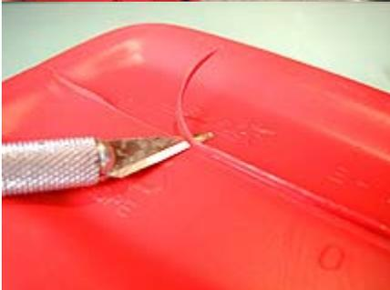
2. After you have dried off the container, take your x-acto knife and trim off the very small seam that resides along the bottom. Removing this seam makes your life much easier when you drill the holes later on.
