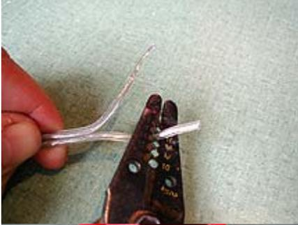
9. Take your lamp cord and strip the end of the wire, removing the plastic sheathing about  $\frac{1}{2}$  inch from the end of the wire. Then, take your fingers and twist the bare wire end to keep all the small wires (which make up the cord) together. Do this for each of the two wires as shown.
