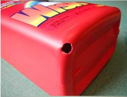
3. Take your 5/16<sup>th</sup> inch drill bit and carefully drill three holes on the bottom edge of the container. Put one hole along the center of the container's side with the handle and then a hole in each corner on the spout side. Sometimes it is easier to use a smaller bit first and then work your way up to the 5/16<sup>th</sup> inch bit.
